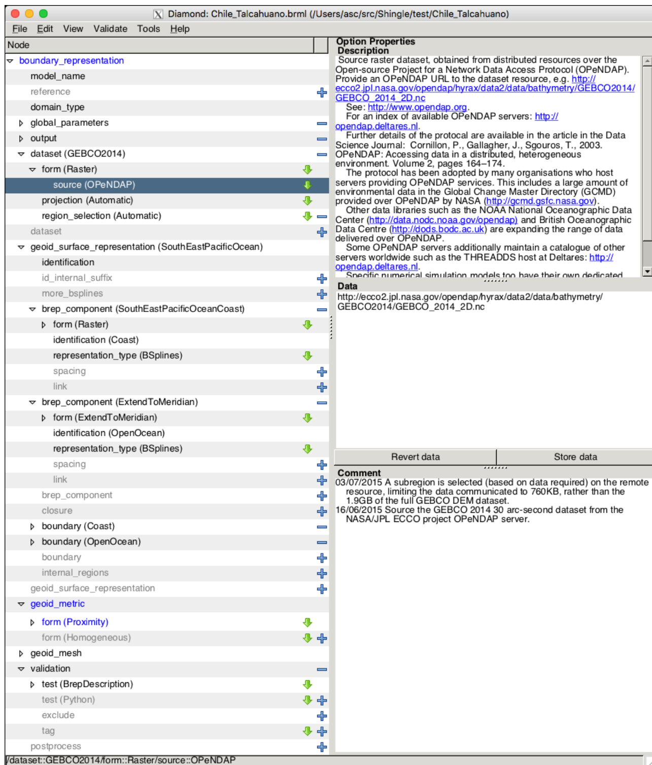
Figure 9.2: An example view of the Graphical User Interface Diamond inspecting the hierarchical tree of option parameters that fully constrain the geophysical domain mesh problem. Each node is shown in context on the left, with their option properties presented on the right, including raw data and the possibility to note comments. This is guided by the BRML schema developed and supplied with Shingle, which additionally provides the fuller self-describing option descriptions shown in the top right. Options down the tree highlighted in blue are mandatory and guide the user to defining a complete set of constraints.
